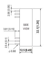
NOTE: Pin tolerance ±0.5mm
