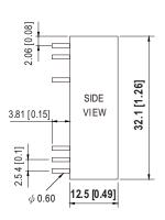
NOTE: Pin tolerance  $\pm 0.5$ mm
