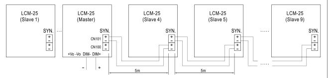
· CN100, CN101: used to synchronously control the LCM units in parallel.
