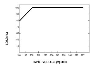
$\frak{\%}$  De-rating is needed under low input voltage.
