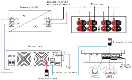
NOTE: After connecting the communication cable, install termination resistors to the remaining sockets of both the ERS-1400 series and CMU2A to prevent signal reflections.
