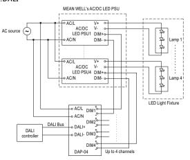
\*Note: Choose a suitable cable for connecting the DAP-04 and DALI controller and make sure the maximum voltage drop between these two units should not be higher than 2V. (Maximum cable length for 1.5mm<sup>2</sup> cables is 300m.)
