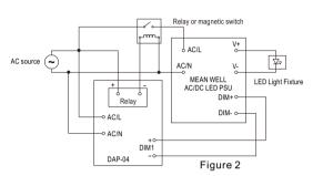
The DAP-04 is equipped with a relay that can be used to turn ON/OFF MEAN WELL LED PSUs. The relay is in the closed position when the DIM1 generates dimming signal; the relay is in the open position when there is no output signal on the DIM1.
