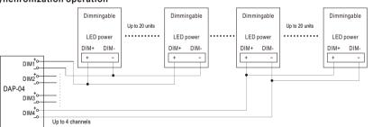
The DAP-04 is equipped with 4 DALI channels, each channel can drive up to 20 LED PSUs, allowing a total of 80 LED PSUs to be connected to the DALI/PWM converter. (Each channel is individually addressable, light intensity of LED PSUs connected to the same channel will be the same; the maximum allowable voltage drop between the DAP-04 and LED PSUs should not be higher than 0.5V; Maximum cable length for 1.31mm<sup>2</sup> cables is 300m.)
